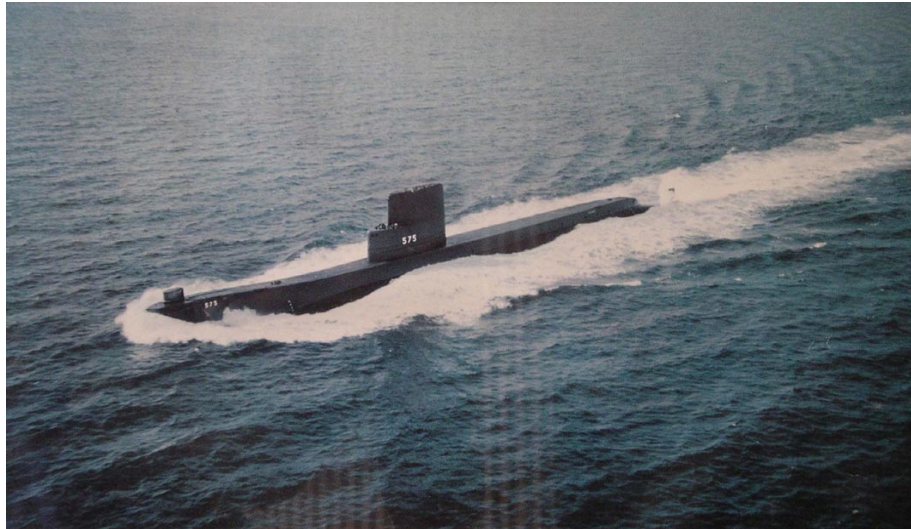
Figure 11. USS Seawolf. The first nuclear submarine powered by a sodium-cooled reactor.
