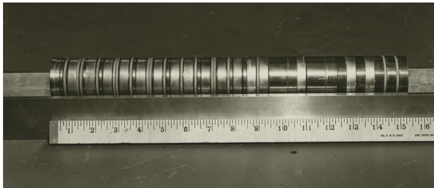
Figure 9. Triflute rod with mounted uranium discs.
